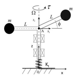
vertical shaft. The shaft rotates with a time varying angular velocity  $\Omega$  with respect to the O<sub>xyz</sub> inertial frame. The arms are of length L. The frame A<sub>x1y1z1</sub> rotates with the arms and attached masses. A time varying torque is applied to the rotor about the z axis, such that  $\tau_{IA} = \tau_o(t)\hat{k}$ . Note that the angle  $\phi$  is fixed.
