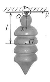
figure. The center of mass is at a distance 'l' from O and  $I_{zz/G}$  is known. An external time varying torque,  $\tau(t)$  is applied to the pendulum at O.
