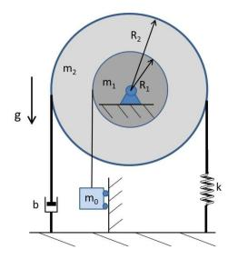
wrapped without slipping around the larger cylinder. The two ends of the string are connected to a spring of constant k on one end and a dashpot of constant b at the other. The smaller cylinder is connected to a block of mass  $m_0$  via an inextensible massless strap, which is wrapped without slipping around the smaller cylinder. The block is constrained to move only vertically.
