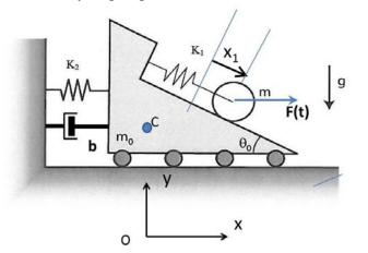
an axel passing through the center of the disk. The cart is also attached to a wall by a spring of constant,  $K_2$ , and a dashpot with constant 'b'. An horizontal external force, F(t), is applied at the center of mass of the disk as shown.
