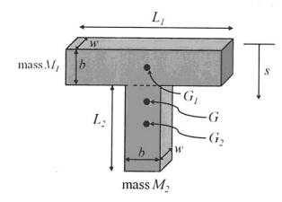
vertical part has length  $L_2$  and mass  $M_2$ .  $G_1$  and  $G_2$  are the centers of mass of each block and are located at the geometric centers of each block.
