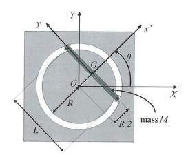
friction. Neglect the mass of the rollers. The radius of the track is R and  $L = \sqrt{3}R$ . Find an equation of motion of the rod as a function of the coordinate,  $\theta$ , as shown in the figure. The frame  $G_{x''y''z'}$  is fixed to the center of mass of the rod.
