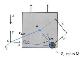
a). In the figure above the point D is the point about which the angular momentum is to be computed. Hence D=A in equations (1) and (2). The point labeled 'B' in the figure is the center of mass for the rigid body and therefore B=G in equations (1) and (2). These are shown in the figure to the left. The rigid body in this case is the combination of the massless pendulum arm and the concentrated mass, M. Also shown in the figure are the position vectors which satisfy the
