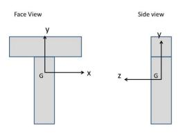
They must be principal axes, because they satisfy the following symmetry properties. The "z" axis is perpendicular to one plane of symmetry. The "x" axis is perpendicular to another plane of symmetry and the "y" axis is perpendicular to x and z.
