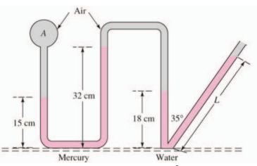
The system above is open to atmospheric pressure  $(10^5 \text{ Pa})$  on its right side.
