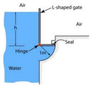
An L- shaped gate can rotate about a hinge pin located at its vertex as shown in the figure above. As the water rises, the depth of the hinge pin, h, will reach a critical height  $h_c$  and the gate will open. If the length of the lower horizontal arm is 1 m, please find the critical height  $h_c$ . (Please neglect the weight of the gate.)
