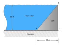
A concrete dam ( $\rho_{concrete}=2500 \text{ kg/m}^3$ ) of triangular cross-section spans 100 m into the page (i.e., the wetted-area of the dam is 100 m (the length of AB) × 100 m (the width into the page) ) in a reservoir as shown above.
