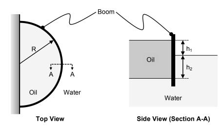
Consider a semi-circular boom of radius R that is deployed to contain oil spill near a dock as shown above. The boom floats on the water and acts as barrier for the spreading oil. The oil has a density  $\rho_o$  and water has density  $\rho_w$  ( $\rho_o < \rho_w$ ). If a volume V of the oil is spilled, calculate:
