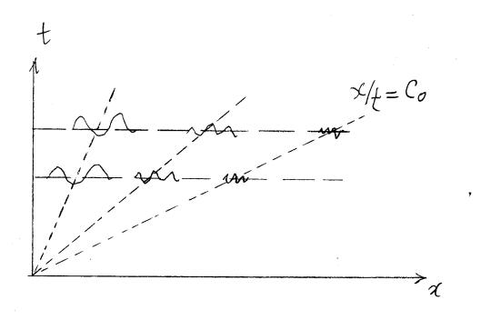
Figure 9: Snapshots of wave field on the side x > 0.
