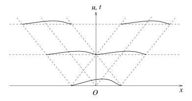
Figure 3: Waves due to initial displacement
