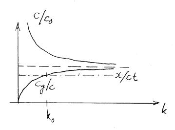
Figure 7: Phase and group velocities of a string in elastic surrounding. Point of Stationary phase  $k_0$ .
