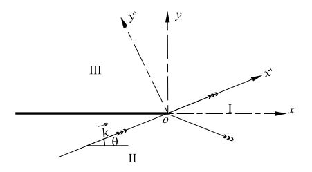
Figure 10: Wave zones near a long crack
