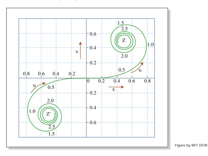
Figure 11: Cornu's spiral, a plot of the Fresnel integrals in the complex plane of  $C(\gamma) + iS(\gamma)$ . Abscissa:  $C(\gamma)$ . Ordinate :  $iS(\gamma)$ .
