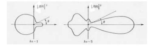
Figure 8: Angular distribution of scattered energy in the far field in cylindrical scattering
