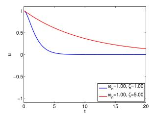
Figure 21.18: Response of overdamped spring-mass-damper systems.
