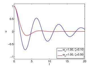
Figure 21.17: Response of underdamped spring-mass-damper systems.
