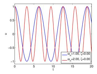
Figure 21.16: Response of undamped spring-mass systems.
