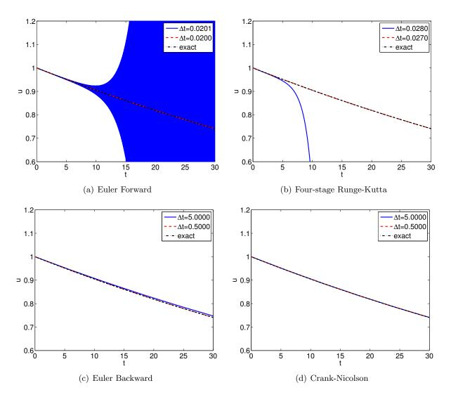
Figure 21.21: Comparison of numerical integration schemes for an overdamped spring-mass-damper system with  $\omega_n = 1.0$  and  $\zeta = 50$ . Note that the time step used for the explicit schemes are different from those for the implicit schemes.
