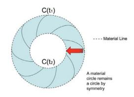
Using Kelvin's Theorem with  $\rho = Const$  and  $\mu = 0$ , and using a circular material line as shown in the figure,
