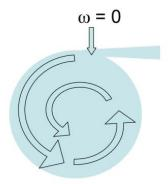
Since the fluid starts with null vorticity  $\omega = 0$ , and  $\frac{D\omega}{Dt} = 0$  (Helmholtz's Vorticity Equation), then it has to remain null as the particle travels through the container, then,
