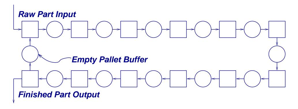
Pallets or fixtures travel in a closed loop. Routes are determined. The number of pallets in the loop is constant.
