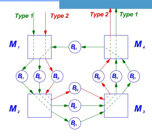
Routes are determined. The number of parts in the loop varies. Semiconductor fabrication is highly reentrant.
