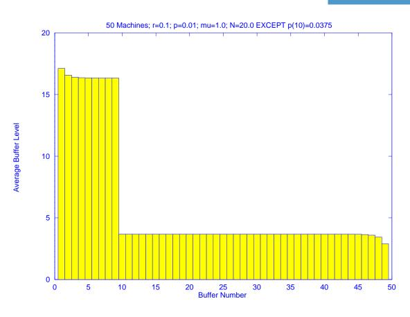
Effect of a bottleneck. Identical machines and buffers, except for  $M_{10}$ .
