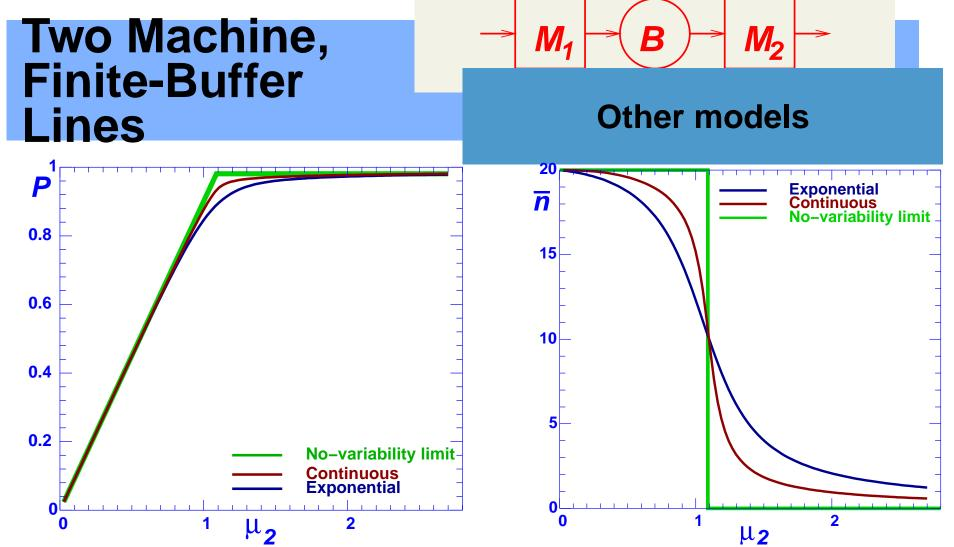
No-variability limit: a continuous model where both machines are reliable, and processing rate  $\mu_i'$  of machine i in the no-variability is the same as the isolated production rate of machine i in the other cases. That is,  $\mu_i' = \mu_i r_i/(r_i + p_i)$ .
