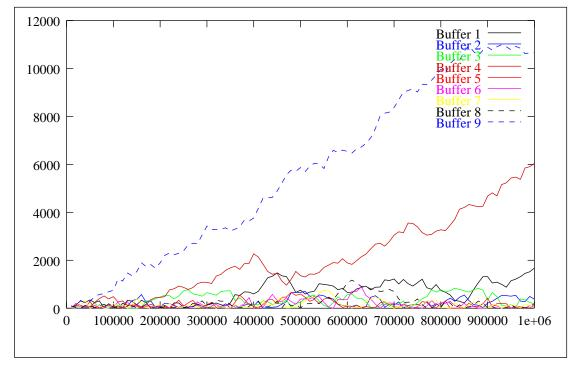
A 10-machine line with bottlenecks at Machines 5 and 10.
