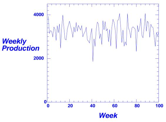
Production output from a simulation of a transfer line.
