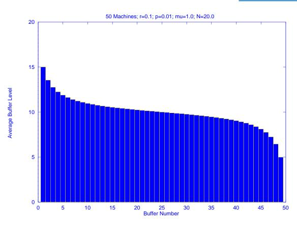
Distribution of material in a line with identical machines and buffers. *Explain the shape.*
