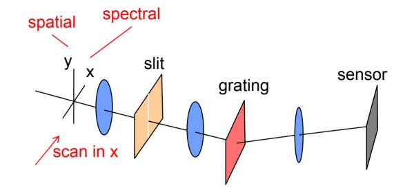
Each row on the sensor provides a spectrum at that y value. Scanning in x provides the other spatial dimension.
