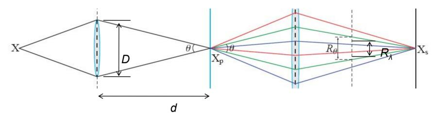
$R_{\theta}$  = width of one wavelength in rainbow plane  $R_{\lambda}$  = distance between centers of extreme wavelengths
