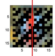
by sliding code over scene vertically (or vice versa) one can mix rows to synthesize columns of uniform scene value.
