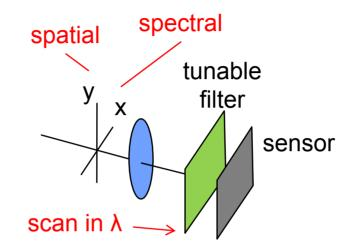
Scan in  $\lambda$  using an electronically-tunable filter. Typically, the filter is based on either liquid crystals or acousto-optic principles.
