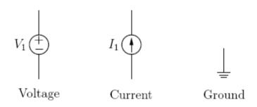
Figure 2: Voltage and Current circuit source symbols, which supply power to circuits. The +, -, and arrow denote voltage polarity and current direction. The ground symbols are defined at the point in the circuit where there is 0V.
