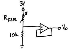
2. For the following circuit, if we want Vo to go from 0V to 5V as the applied force goes from 0kg to 1kg, what value should R be?
