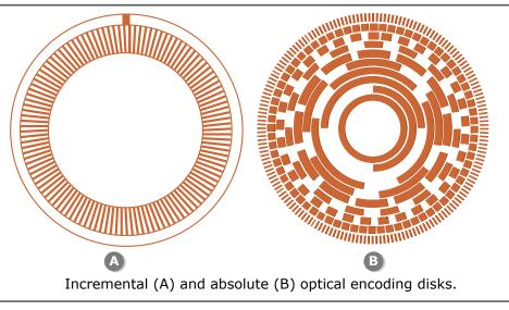
Image by MIT OpenCourseWare. (L) Incremental and (R) optical encoding disks.
