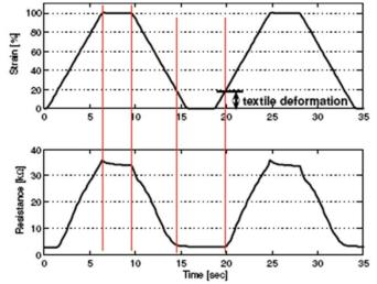
Figure 3. Typical response of sensor to a given strain (sensor length 2cm).
