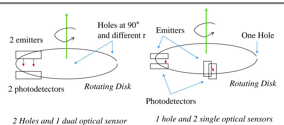
One sensor measures "I" and the other measures "Q" -> Direction determined by whether I leads Q in time or vice-versa *Can be spaced more closely, for rapid direction determination*
