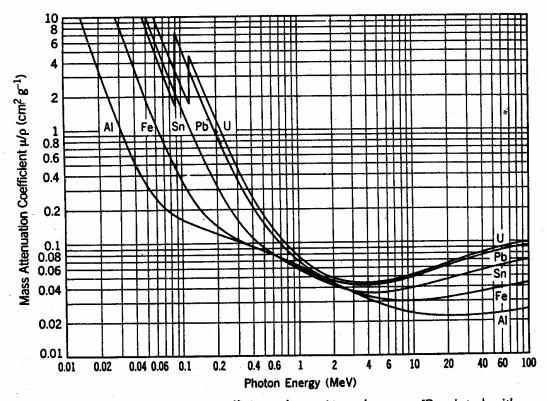
FIGURE 8.8. Mass attenuation coefficients for various elements. [Reprinted with permission from K. Z. Morgan and J. E. Turner, eds., *Principles of Radiation Protection*, Wiley, New York (1967). Copyright 1967 by John Wiley & Sons.]
