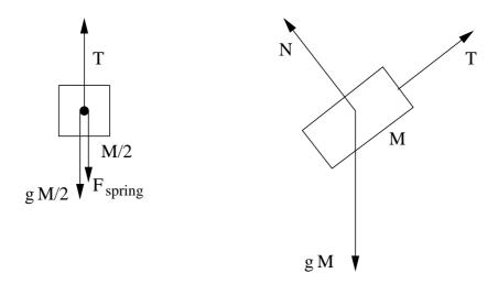
(b) Assume the potential energy is zero when the string is unstretched. After we pull the M block by a distance L, the potential energy of the M block is lower by  $MgL\sin\theta$ , the potential energy of the M/2 block is increased by  $\frac{M}{2}gL$ , and the potential energy of the spring is increased by  $\frac{1}{2}kL^2$ . So the total potential energy of the system is
