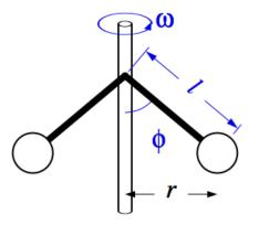
a) Describe the acceleration of the spheres. Explaining and quantifying your knowledge of the acceleration will help you model the problem. Show all relevant free body diagrams.
