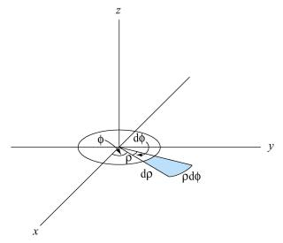
Figure 9.2.8 Area element for a disc
