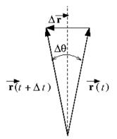
Figure 9.3 Change in position vector for circular motion.
