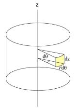
Figure 9.2.7 Area element for a cylinder
