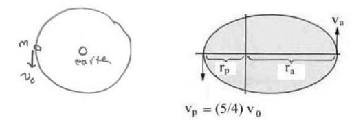
As a result of a satellite maneuver, the satellite trajectory is changed to an elliptical orbit. This is accomplished by firing a rocket for a short time interval and increasing the tangential speed of the satellite to  $(5/4)v_0$ . You may assume that during the firing, the satellite does not noticeably change the distance from the center of the earth.
