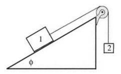
a) What is the relation between the masses of block 1 and block 2 such that the system just starts to slip?
