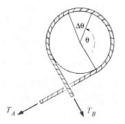
The load on the rope pulls it with a force  $T_A$ , and the sailor holds the other end of the rope with a much smaller force  $T_B$ . The coefficient of static friction between the rope and the drum is  $\mu_s$ . The sailor is holding the rope so that it is just about to slip. Can you show that  $T_B = T_A e^{-\mu_s \theta}$ , where  $\mu_s$  is the coefficient of static friction and  $\theta$  is the total angle subtended by the rope on the drum?
