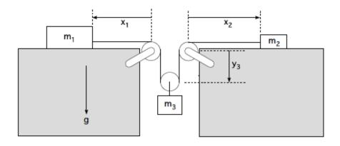
In the system shown above  $m_1 > m_2$ . The pulleys are massless and frictionless, and the rope joining the blocks has no mass. The coefficient of static friction between the blocks and the tables is greater than the coefficient of kinetic friction:  $\mu_s > \mu_k$ . The downward acceleration of gravity is g.
