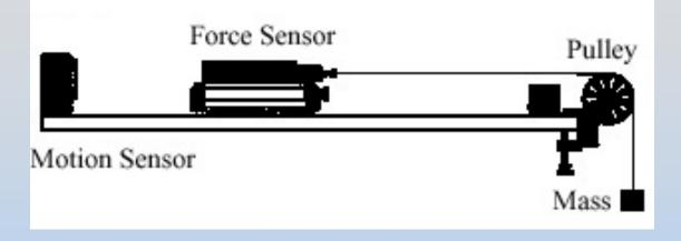
Consider a track with a pulley located at one end. The force sensor and cart have total mass  $m_1$ . They are connected by an inextensible rope of length *I* (passing over the pulley) to a block of mass  $m_2$ . You may ignore the small mass of the rope and pulley. You may also assume that all friction effects are negligible. What is the tension in the string both before the cart is released and while the cart is in motion?
