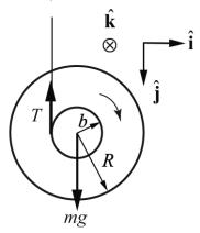
The direction of the torque is into the page in the figure above (positive z-direction). Use the right-hand rule to check this, or use the cross-product definition of torque:
