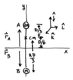
The center of mass is a distance (2/3)D from the object at B and is a distance (1/3)Dfrom the object at A.
