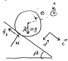
Choose x = 0 as the point where the cylinder just starts to roll. With the unit vectors shown in the figure above, Newton's Second Law, applied in the x- and y-directions in turn, yields
