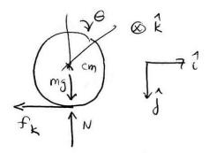
At t = 0, when the ball is released,  $\vec{\mathbf{v}}_{cm,0} = v_0 \hat{\mathbf{i}}$  and  $\vec{\boldsymbol{\omega}}_0 = \vec{\mathbf{0}}$ , so the wheel is skidding and hence the friction force on the wheel due to the sliding of the wheel on the surface opposes the motion is kinetic friction and hence acts in the negative  $\hat{\mathbf{i}}$ -direction.
