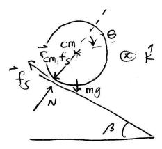
Then, the only force exerting a torque about the center of mass is the friction force, and so we have
