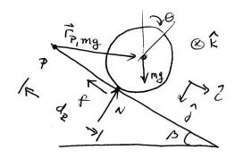
The gravitational force  $M\vec{\mathbf{g}} = Mg\sin\beta \hat{\mathbf{i}} + Mg\cos\beta \hat{\mathbf{j}}$  acts at the center of mass. The vector from the point P to the center of mass is given by  $\vec{\mathbf{r}}_{P,mg} = d_P \hat{\mathbf{i}} - R \hat{\mathbf{j}}$ , so the torque due to the gravitational force about the point P is given by
