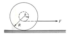
The coefficient of static friction between the Yo-Yo and the table is  $\mu_s$ .
