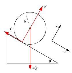
b) With the coordinates system shown, Newton's Second Law, applied in the x - and y - directions in turn, yields
