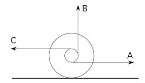
Two disks are separated by a spindle of smaller diameter. A string is wound around the spindle and pulled gently. At what position of the string does the direction of rotation change?
