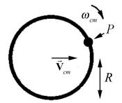
Consider a wheel of radius *R* is rolling in a straight line. The center of mass of the wheel is moving in a straight line at a constant velocity  $\vec{\mathbf{V}}_{cm}$ . Let's analyze the motion of a point *P* on the rim of the wheel.
