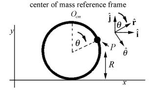
Now substitute Eqs. (26.3.2) and (26.3.6) into Eq. (26.3.1) for the velocity of a point P on the rim in the reference frame fixed to the ground
