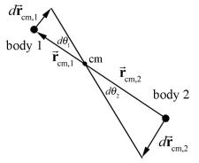
Figure 26.A.3: infinitesimal angular displacements in the center of mass reference frame
