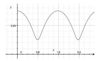
This path is called a *cycloid*. We can differentiate the position vector in the reference frame fixed to the ground to find the velocity of the bead
