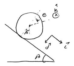
For a time interval  $\Delta t$ , the displacement of the center of mass is given by  $\Delta \vec{\mathbf{R}}_{cm}(t) = \Delta X_{cm} \hat{\mathbf{i}}$ . The arc length due to the angular displacement of a point on the rim during the time interval  $\Delta t$  is given by  $\Delta s = R\Delta\theta$ . The rolling without slipping condition is
