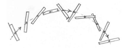
Figure 26.1 The center of mass of a thrown rigid rod follows a parabolic trajectory while the rod rotates about the center of mass.
