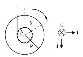
Consider a point on the rim of the axle at a distance r = b from the center of mass. As the yo-yo falls, the arc length  $\Delta s = b\Delta\theta$  subtended by the rotation of this point is equal to length of string that has unraveled an amount  $\Delta l$ . In a time interval  $\Delta t$
