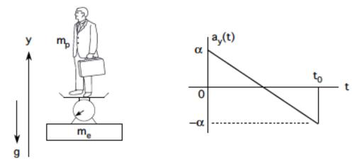
A person of mass  $m_p$  stands on a scale in an elevator of mass  $m_p$ . The scale reads the magnitude of the force F exerted on it from above in a downward direction. Starting at rest at t = 0 the elevator moves upward, coming to rest again at time  $t = t_0$ . The downward acceleration of gravity is g. The acceleration of the elevator during this period is shown graphically above and is given analytically by
