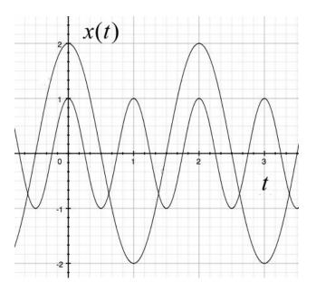
The multiplying factor A is known as the *amplitude* (the amplitude is, strictly speaking, is |A|). The function x(t) assumes values between -|A| and |A|. The constant T has dimensions of time, and is known at the *period* of the oscillation. For the purposes of this problem (and many similar problems), a function x(t) has *periodicity* T if
