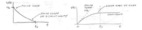
We shall first find the acceleration and then integrate the acceleration to find an equation for how the horizontal component of the velocity varies with time. We shall use this equation to find the time that the plane comes to a stop since the horizontal component of the velocity is zero at that instant. Then we shall use the position equation to determine how far the airliner has traveled before it came to a stop.
