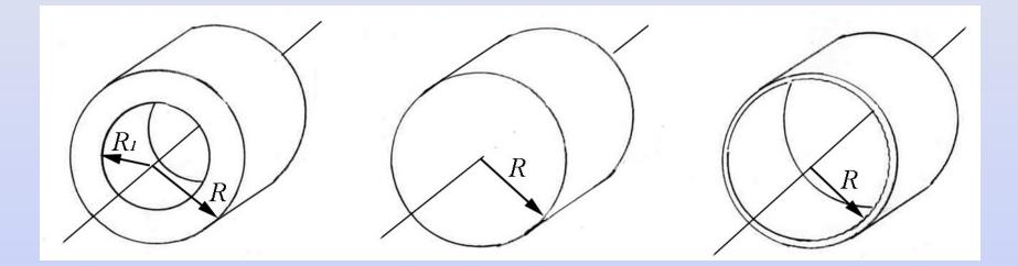
1) Hollow Cylinder 2) Solid Cylinder 3) Thin-walled Hollow Cylinder
