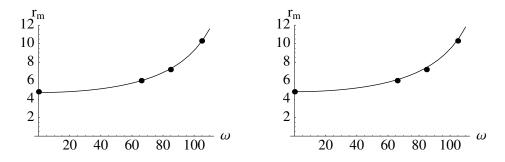
Figure 3: The one and two-parameter fits. Left: two-parameter fit.  $A = 4.7 \, cm$ ,  $\omega_c = 143 \, s^{-1}$ , RMSE is  $0.07 \, cm$ . Right: one-parameter fit,  $\omega_c = 144 \, s^{-1}$ , RMSE is  $0.14 \, cm$ .
