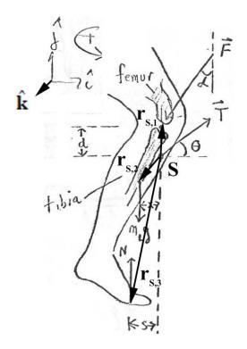
Choose the point of action of the ligament on the femur as the point *S* to compute the torque about. Note that the tensile force,  $\vec{T}$ , that the ligament exerts on the upper tibia will make no contribution to the torque about this point *S*. Choose counterclockwise c as the positive direction for the torque, this is the positive  $\hat{k}$  direction. Then the torque due to the force of the femur  $\vec{F}$  on the tibia is
