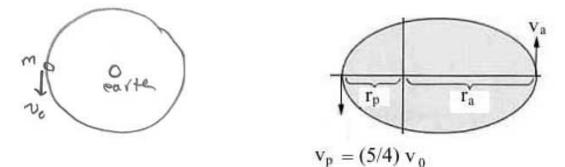
As a result of a satellite maneuver, the satellite trajectory is changed to an elliptical orbit. This is accomplished by firing a rocket for a short time interval and increasing the tangential speed of the satellite to  $(5/4)v_0$ . You may assume that during the firing, the satellite does not noticeably change the distance from the center of the earth.
