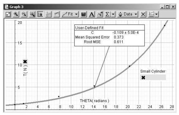
The fit gave  $\mu = 0.11$ , in good agreement with the result for the large cylinder. (Again, the Natural Exponent Fit worked, but the parameter values were unreasonable, a case of too many fit parameters for somewhat noisy data being a bad thing.)
