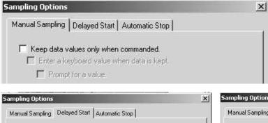
On the Manual Sampling tab of the Sampling Options window that opens, make sure that none of the boxes are checked. Set the delayed start to none, and automatic stop to 10 s.
