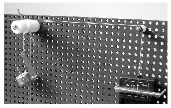
Use the same apparatus as for the static equilibrium experiment, but remove the sliding T-square and attach the plastic cylinder near the top center of the board. The cylinder has a handle so you can turn it and two regions for wrapping the string. One has a diameter of 0.5 in and the other of 1.0 in. You may use either one, but discuss with the other groups at your table to make sure that both diameters are being used at your table.
