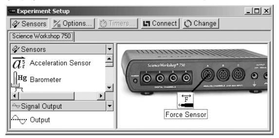
Drag the force sensor icon to the interface in the Experiment Setup window. Double-click the force sensor icon to open a window to set the Sensor Properties. Under the "General" tab, choose a sample rate of 10 Hz, and "Slow Force Changes (Spring Tests)". Under the "Calibration" tab, choose Sensitivity: "Low (1x)". (The force sensor records force as a negative number when you pull on it.)
