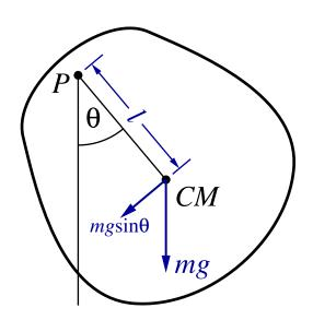
For the ideal pendulum the tangential restoring force is  $mg\sin\theta$  and the displacement is  $l\theta$ , giving rise to the equation of motion (F = ma)
