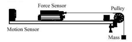
A force sensor on a cart is attached via a string to a hanging weight. The cart is initially held. When the cart is allowed to move does the tension in the string
