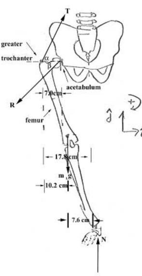
You would like to compute the magnitude of the tension of the hip abductor muscles. About which point should you calculate the torque?
