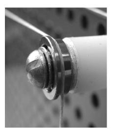
Increase ccw torque on cylinder smoothly to the slipping point, then turn slowly for 1 or 2 seconds. Practice this, so you get 1 or 2 peaks of the force in 10 s, then record the force with *DataStudio*.
