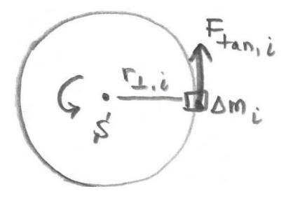
$$\tau_{S,i} = r_{\perp,i} F_{\tan,i} = \Delta m_i (r_{\perp,i})^2 \alpha$$
