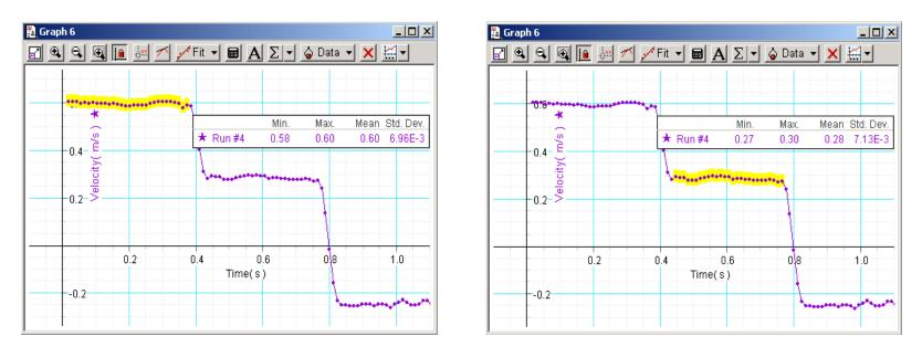
$\Box$  Use Statistics Tool ( $\Sigma$ ) to measure velocities  $v_{\mathcal{A},1}$  and  $v_2$ , before and after
