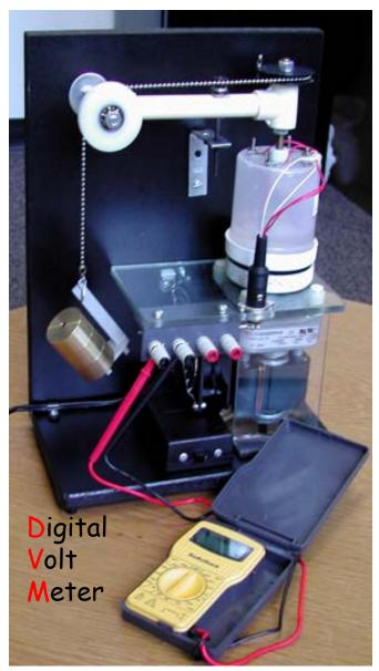
Mechanical equivalent to heat: A motor applies a known friction motor applies a known  $\omega$  to a plastic  $c = \frac{f}{m(dT/dt)}$
