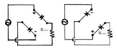
Figure 8: Bridge rectifier in action
