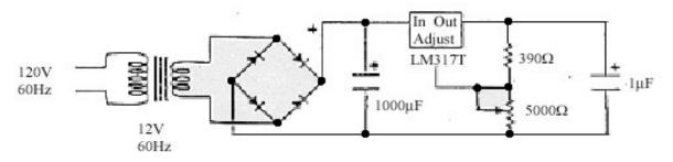
Figure 2: Circuit diagram for LVPS
