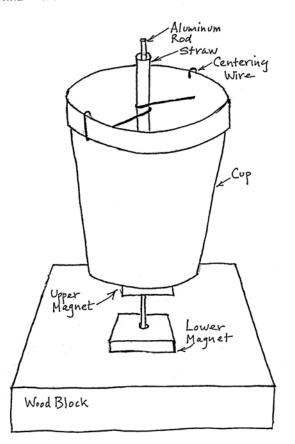
To make sure the apparatus is OK, press down on the cup with two fingers on a diameter until the magnets touch and release it—the cup should bounce up and down about 3 or 4
