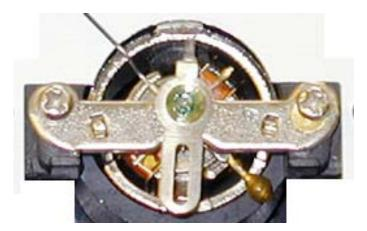
**Figure 2: Multimeter Coil**
