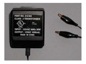
Figure 3: Wall transformer
