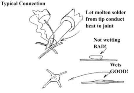
**Figure 2: Soldering Connections**
