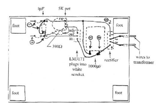
Figure 19: Wiring on bottom side of LVPS
