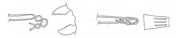
Figure 2: Wiring Nuts
