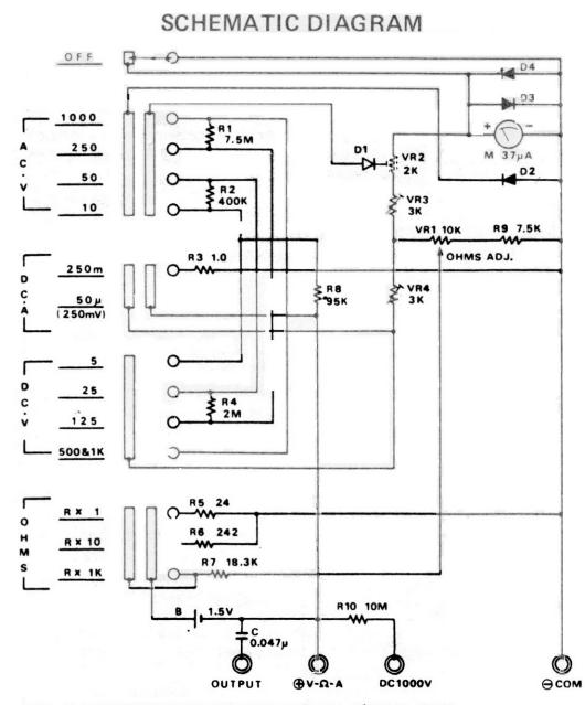
NOTE: (1) ALL RESISTANCE VALUES ARE INDICATED IN "OHM" (K =  $10^{3}$  OHM, M =  $10^{5}$  OHM) (2) ALL CAPACITANCE VALUES ARE INDICATED IN " $\mu$ F" (P =  $10^{-5}\mu$ F);
