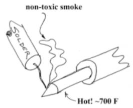
Figure 1: Tinning the soldering iron
