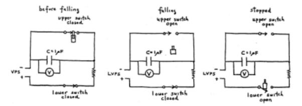
Figure 1: Circuit diagrams for falling object
