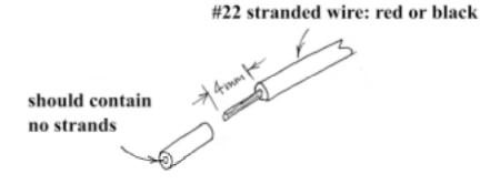
Figure 3: Stripping wires
