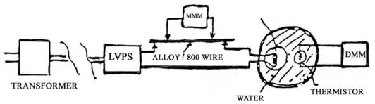
**Figure 4: Circuit Diagram for Experiment ET**
