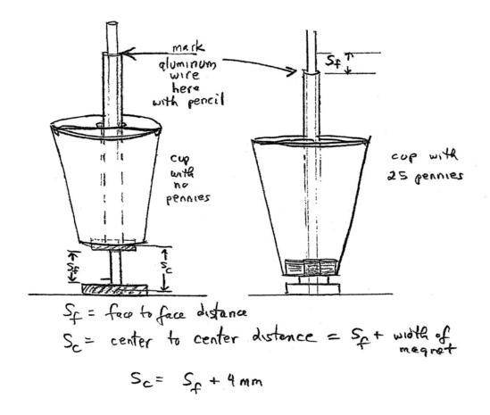
• Place the upper magnet and cup on the wire. The magnets are now closer because of the weight of the cup, straw and centering wire,  $0.025 \pm 0.003$  N. Make a pencil mark on the aluminum wire next to the top of the straw.
