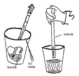
Figure 2: calibrating the Thermistor
