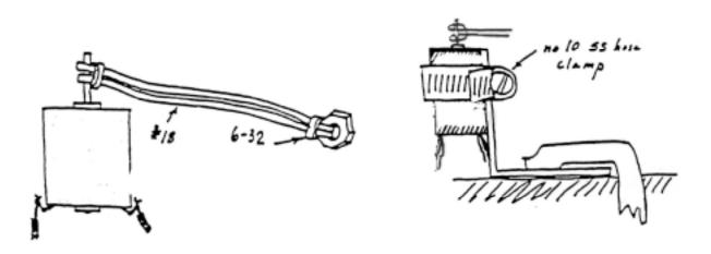
Figure 2: Clamping the motor and attaching the nut
