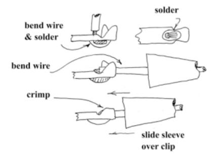
Figure 5: Soldering clip leads
