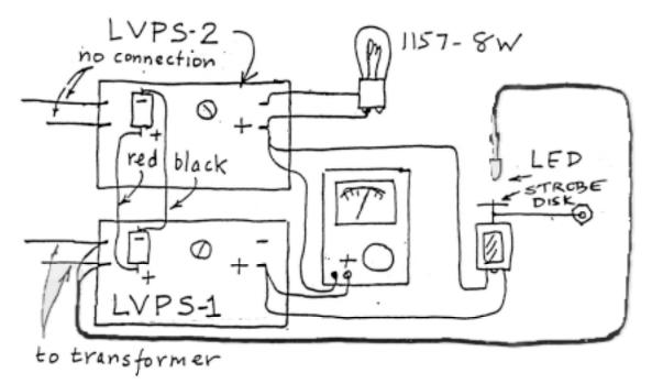
**Figure 3: Connecting the two LVPS**
