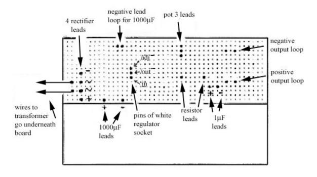
Here is a template (top view) to help place the parts on the perfboard.
