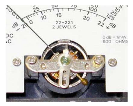
Figure 1: Coil and torsion spring
