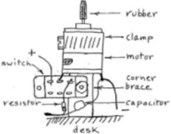
Figure 3: Hookup diagram for DPDT
