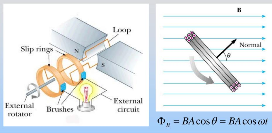
$$\mathcal{E} = -N\frac{d\Phi_B}{dt} = -NAB\frac{d}{dt}(\cos\omega t) = NAB\omega\sin\omega t$$
