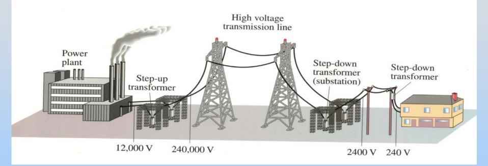
Power loss can be greatly reduced if transmitted at high voltage
