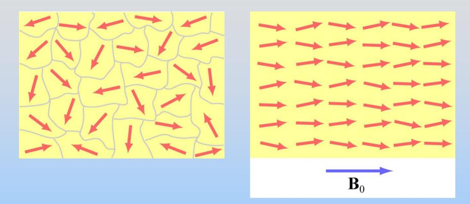
Applied external field B<sub>0</sub> tends to align the atomic magnetic moments
