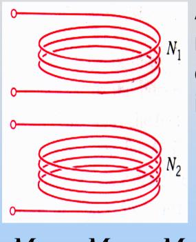
A current  $I_2$  in coil 2, induces some magnetic flux  $\Phi_{12}$  in coil 1. We define the flux in terms of a "mutual inductance"  $M_{12}$ :
