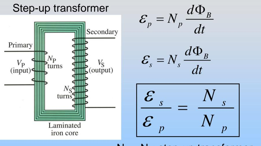
$N_s > N_p$ : step-up transformer  $N_s < N_p$ : step-down transformer <sub>P21- 26</sub>
