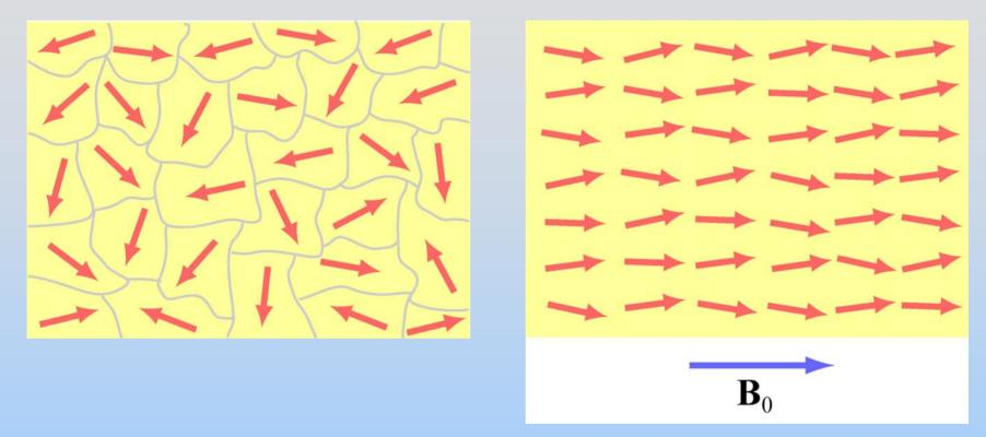
Paramagnet: Turn off  $B_0$ , everything disorders Ferromagnet: Turn off  $B_0$ , remains (partially) ordered
