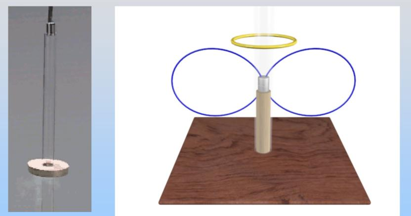
Falling magnet approaches a copper ring or Copper Ring approaches Magnet P21- 6
