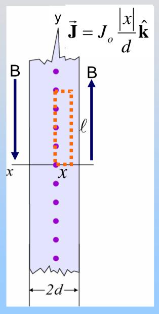
Direction: Up on right, down on left Inside: (at 0<x<d):  $\oint \vec{\mathbf{B}} \cdot d\vec{\mathbf{s}} = \mu_0 I_{enc}$  $\oint \vec{\mathbf{B}} \cdot d\vec{\mathbf{s}} = B\ell + 0 + 0 + 0$  $\mu_0 I_{enc} = \mu_0 \iint \vec{\mathbf{J}} \cdot d\vec{\mathbf{A}} = \mu_0 \int_0^x \frac{J_0 x}{d} \ \ell dx$  $=\mu_0 \frac{J_0 \ell}{d} \frac{x^2}{2}$
