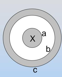
Consider a coaxial cable of with inner conductor of radius *a* and outer conductor of inner radius *b* and outer radius *c*. A current *I* flows into the page on the inner conductor and out of the page on the outer conductor.
