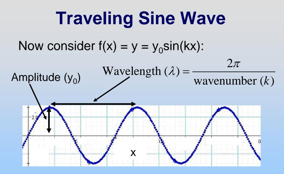
What is g(x,t) = f(x+vt)? Travels to left at velocity v  $y = y_0 sin(k(x+vt)) = y_0 sin(kx+kvt)$  **Traveling Sine Wave**  $y = y_0 \sin(kx + kvt)$
