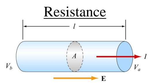
When a current flows in a wire of length *L* and cross sectional area *A*, the resistance of the wire is
