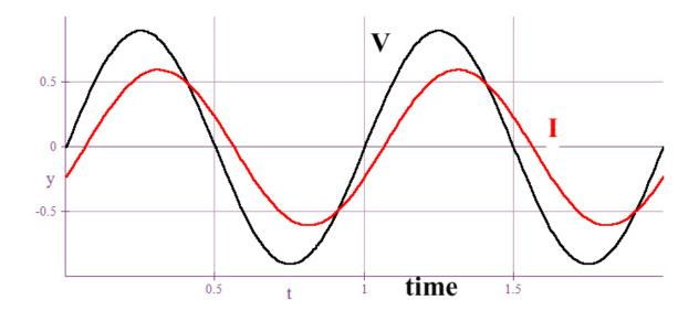
The plot shows the driving voltage V (black curve) and the current I (red curve) in a driven RLC circuit. In this circuit,
