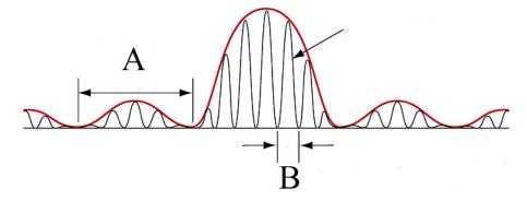
Coherent monochromatic plane waves impinge on two long narrow apertures (width a) that are separated by a distance d (d >> a). The resulting pattern on a screen far away is shown above. Which structure in the pattern above is due to the finite width a of the apertures?
