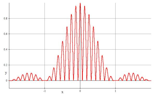
Coherent monochromatic plane waves impinge on two long narrow (width *a*) apertures separated by a distance *d*. The resulting pattern on a screen far away is shown above. For this arrangement:
