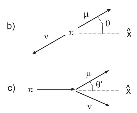
Figure 4: Decay of a pion to a muon and neutrino: a) Decay in pion rest frame. Since the total momentum is zero, the neutrino and muon have equal and opposite momenta. b) Pion decay in pion rest frame. The muon momentum makes an angle  $\theta$  with the x axis. c) Decay of a pion moving along the x axis. In this frame, the muon momentum makes an angle  $\theta'$  with the x axis.
