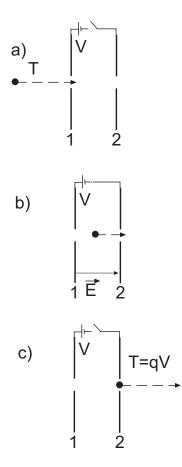
Figure 1: Acceleration of a particle. a) A particle with velocity close to c approaches a set of parallel plates. b) When the particle passes plate 1, a potential V is turned on, creating a field E which exerts a force F=qE on the particle. c) When the particle leaves the plates, the potential is turned off. The particle now has qV more kinetic energy than before, regardless of its initial velocity.
