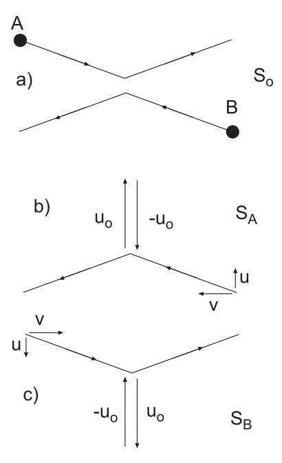
Figure 2: Scattering experiment. a. In frame  $S_o$ , the particles A and B collide with equal and opposite momenta. b. In  $S_A$ , particle A moves only along the  $\hat{y}$  axis. c. In  $S_B$ , particle B moves only along the  $\hat{y}$  axis. Frame  $S_B$  moves in the  $-\hat{x}$  direction with velocity v with respect to frame  $S_A$ .
