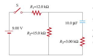
(a) Find the steady-state current in each resistor.
