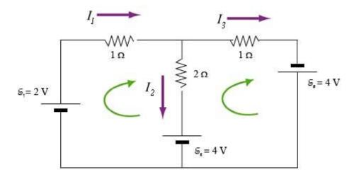
Current conservation is given by the condition that the current into a junction of branches is equal to the current that leaves that junction:
