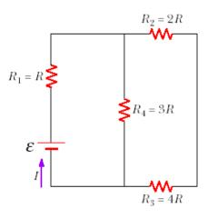
$$\Delta V_1 = \frac{\varepsilon}{3}, \quad \Delta V_2 = \frac{2\varepsilon}{9}, \quad \Delta V_3 = \frac{4\varepsilon}{9}, \quad \Delta V_4 = \frac{2\varepsilon}{3}$$
