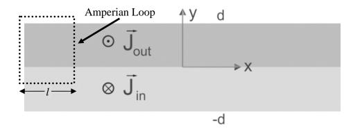
c) Use Ampere's Law to find the magnetic field for 0 < y < d. Show the Amperian Loop that you use and give the magnitude and direction of the magnetic field.
