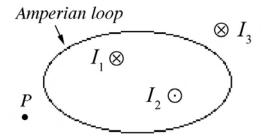
Which currents produce the magnetic field at the point *P* shown in the sketch (circle one)?
