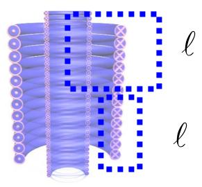
The loop has four segments. Along two of those (top and bottom, horizontal),  $\vec{\bf B}$  is perpendicular to  $d\vec{\bf s}$ , and  $\vec{\bf B}\cdot d\vec{\bf s}=0$ . On the other hand, along the outer vertical segment,  $\vec{\bf B}=0$ . Thus, using Ampere's law  $\oint \vec{\bf B}\cdot d\vec{\bf s}=\mu_0 I_{\rm enc}$ , we have
