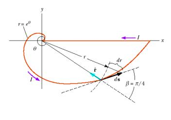
To complete a loop, the ends of the spiral are connected by a straight wire along the *x* axis. Find the magnitude and direction of  $\vec{\mathbf{B}}$  at the origin.
